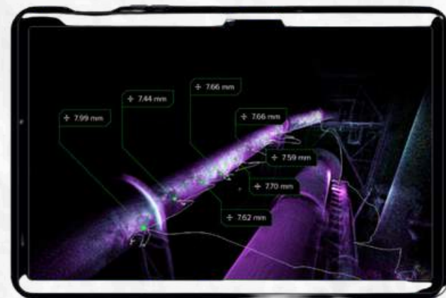
Flyability - Elios 3 UT / Ultrasonic Test: Thickness Analysis
